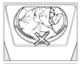
Check the laundry is right inside the drum so that it cannot get trapped or damaged when the door is shut.
